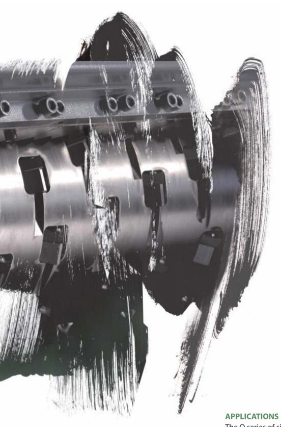
The Q series of single shaft shredders are suitable for processing almost all plastics. The machines will shred production waste, pipes, automotive parts, blow-moulded materials such as PET-bottles, PE/PP bottles, containers or buckets. Moreover, materials such as wood, paper, cardboard can be shredded without problems.
